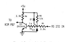
Figure 3: One transistor buffered by resistors and diodes makes an RS-232 input port with protection against unexpected voltages.
